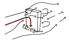
Fig. 1 An illustration of typical airflow conditions around a rectangular building (drawn by the author).
