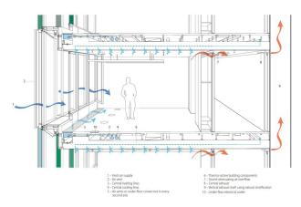
Fig. 21 Detailed section of typical office ventilation © Sauerbruch Hutton.
