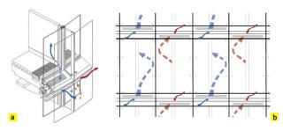
**Fig. 7** Isometric drawing of the double-skin façade illustrating the Fish Mouth device (a); and façade elevation showing the alternating system of the inlet and outlet modules (b) © Ingenhoven architects.
