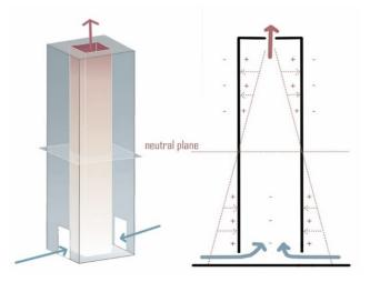
Fig. 3 Illustration of buoyancy induced ventilation in the absence of the wind for a rectangular tall building (drawn by the author).
