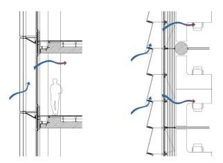
Fig. 19 Detailed section through the double-skin façade (a), detailed plan through the double-skin façade (b) © Sauerbruch Hutton.
