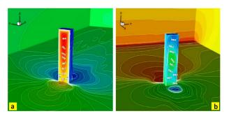
Fig. 2 Distribution of mean pressure coefficient over the building walls at the windward side (a); and the leeward side (b) (Braun and Awruch, 2009).
